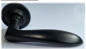
A deep matt black chromium plating on top of a specially prepared surface producing a flat non-reflective finish. Chromium plating is a very hard wearing, stable finish, suitable for most environments. An occasional light application of a good quality wax will assist in keeping the finish in good condition. Metal polish can be used if desired.
