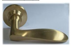
A satin polished solid brass surface treated with a thin beeswax coating for protection during transit and installation. An unlacquered living finish, intended to oxidize and patina naturally over time. An occasional light application of a good quality wax will assist in keeping the finish in good condition.
