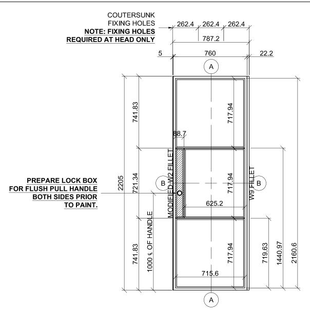
1No. REQUIRED. KITCHEN - GROUND FLOOR - INTERNAL. VIEWED FROM KITCHEN. SUPPLY ONLY - EC1 CONSTRUCTION TO INSTALL ON SLIDING TRACK SYSTEM.
